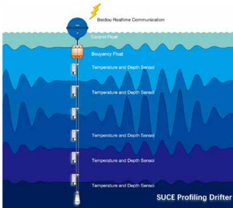
SUCE Profiling Drifter in the application of real time monitoring on internal waves
