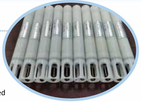
The Ocean Observation Technology and Data Center (OOTDC) developed a self-contained *in situ* sea water temperature logger in 2023. This instrument has the advantages of high precision, small size, is easy to operate, and is low cost. As a widely used instrument for *in situ* observations, it can be incorporated into various observation systems, including ocean buoys, subsurface moorings, and seabed-based platforms, to acquire time series of sea water temperature distribution and variations.
